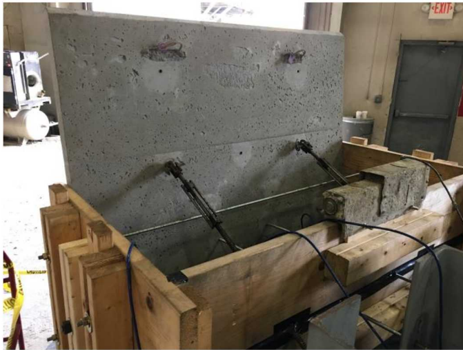
Figure 3: Test Panel with Deck Pour Containment Form
