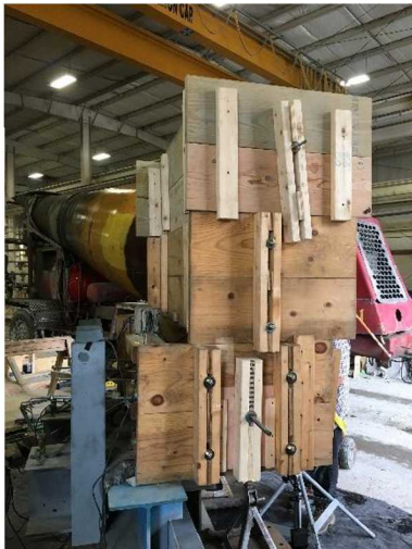
Figure 3: Test Panel with Deck Pour Containment Form Figure 4: Load Media Being Weighed
