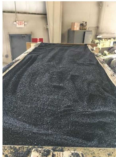
Figure 6: Test panel with Completed Overpour Load Condition
