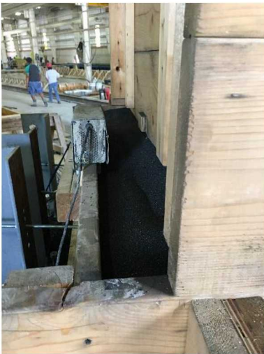
Figure 5: Test Panel with Completed Deck Pour Load Condition
