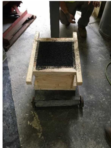
Figure 3: Test Panel with Deck Pour Containment Form Figure 4: Load Media Being Weighed
