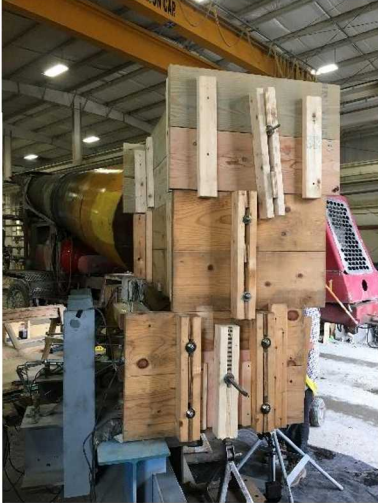
Figure 3: Test Panel with Deck Pour Containment Form
