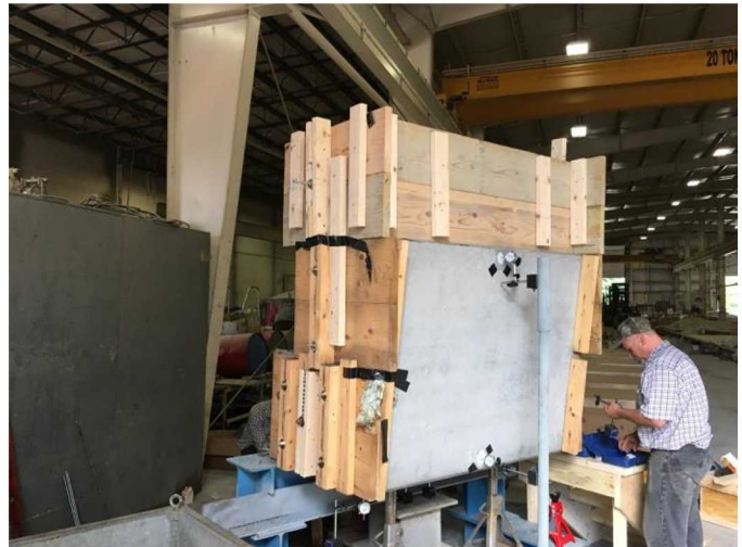
Figure 6: Test Panel with Containment Forms for all Load Cases
