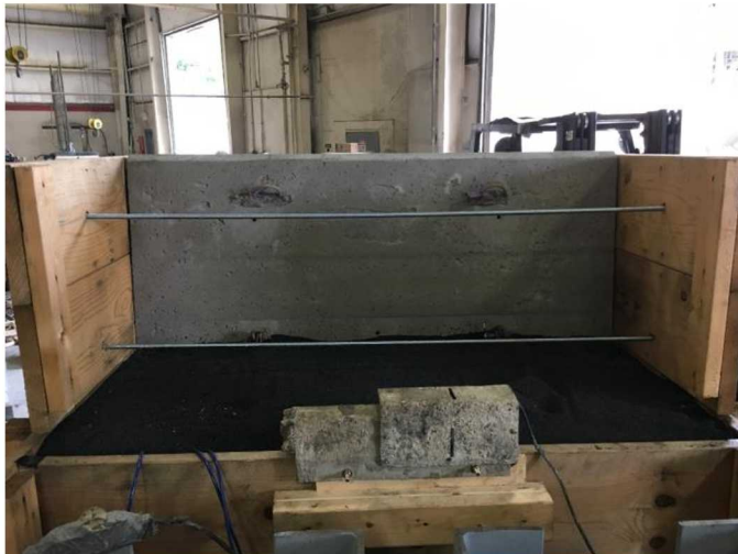
Figure 5: Test Panel with Completed Deck Pour Load Condition
